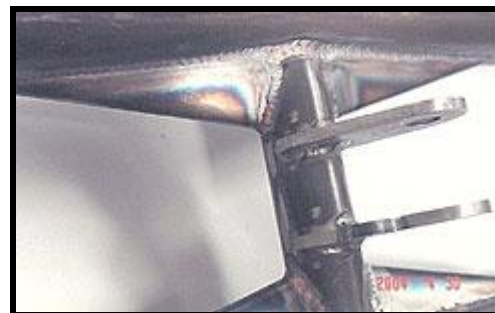
Top quality TIG welded joints
