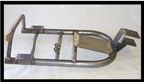
Yamaha Golf Cart swingarm Allows 24 HP Honda bolt in conversion.
