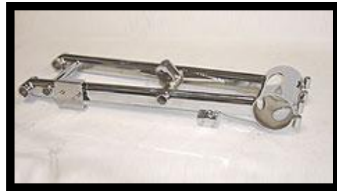
TRX450 Swingarm Shown with optional chroming. Oval tube model. (Square tube also available) $429.00
