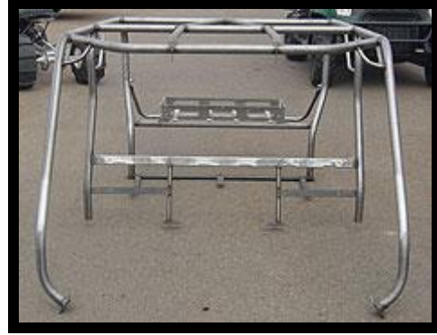
Polaris Ranger (full cage) Includes seat mounting tabs reclines back rest for more comfort.
