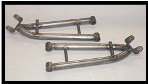
A-Arms to lift Yamaha Golf cart Using original A-Arm mounting pts. We use either stock or longer shocks.
