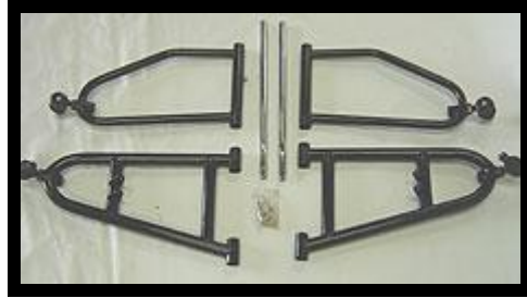
YFZ 450 A-Arms Shown in bare metal +2"/+1" configuration. $460.00
