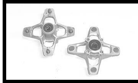
Stock Banshee Front Hubs CNC milled for weight and appearance. $50.00 / pair
