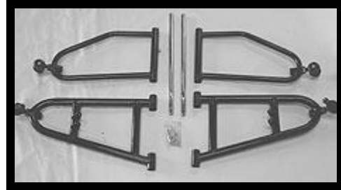
YFZ 450 A-Arms Shown in bare metal +2"/+1" configuration. $460.00
