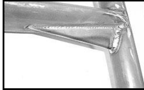
Top quality TIG welded joints
