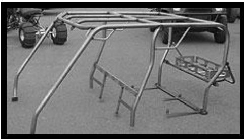
Polaris Ranger (full cage) Includes seat mounting tabs reclines back rest for more comfort.
